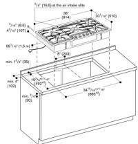
Minimum distance from the appliance cut-out to the side wall  $11^{10}(390 \ \text{mm})$ .
